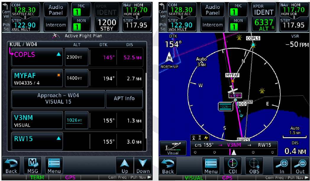
Figure 3: Flight plan setup (view at departure) and final descent segment with “Vertical Speed Required” (VSR) in a Garmin GTN750 unit, as configured per the scenario of Question 6.
