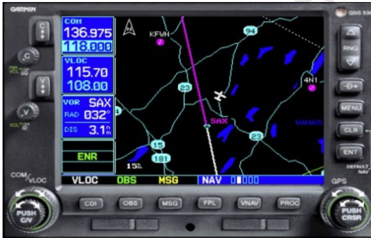
Figure 6: Distance and bearing from the Sparta (SAX) VOR station as displayed by a Garmin GNS530 GPS unit.
