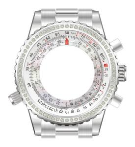
When these two rings match, you have a ratio of 1:1. So now rotate the number 30 on the outer scale so that it is in line with the red 60 on the middle scale. 30 is half of 60 so you have now just created a ratio of 2:1 (two "30s" equal one "60"). Notice that 35 is over 70 and 40 is over 80. You will use these ratios
