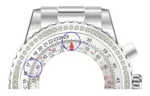
Now you can also find out other information using this example. Let's say your fuel burn rate is 26 gph (gallons per hour) and you want to find out how long you could get on a full tank of usable fuel. If a full tank of gas was equal to 140 gallons (which you should know if you are flying a plane that has a maximum useable fuel of 140 gallons), then here is how you would find your *endurance*.
