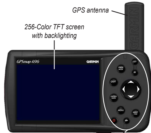
Backlit keypad for easy nighttime operation
