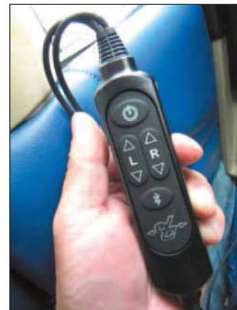
The rest-on-ear supra-aural cups on the DC Pro-X make the headset sunglasses-friendly, top photo. The feed-forward/feedback noise-canceling circuitry uses dual noise-sampling microphones that are mounted in each ear cup, middle photo. The control module, bottom photo, has good ergonomics but a fragile battery lid.
